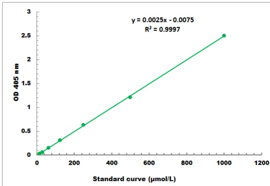
Detection Range: 10  $\mu\text{mol/L}$  - 1000  $\mu\text{mol/L}$
