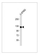
Anti-CSF1R Antibodyat 1:4000 dilution + U-87MG whole cell lysates Lysates/proteins at 20 µg per lane. Secondary Goat Anti-mouse IgG, (H+L), Peroxidase conjugated at 1/10000 dilution Predicted band size : 108 kDa Blocking/Dilution buffer: 5% NFDM/TBST.
