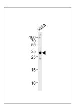
Western blot analysis of lysate from HeLa cell line, using RPS6 Antibody (N-term)(Cat. #AP1977a). AP1977a was diluted at 1:1000 at each lane. A goat anti-rabbit IgG H&L(HRP) at 1:5000 dilution was used as the secondary antibody. Lysate at 35ug per lane.
