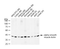
25 ug total protein per lane of various lysates (see on figure) probed with alpha smooth muscle Actin polyclonal antibody, unconjugated (AP50856) at 1:2000 dilution and 4°C overnight incubation. Followed by conjugated secondary antibody incubation at r.t. for 60 min.
