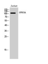
Western Blot analysis of Jurkat cells using GPRC6A Polyclonal Antibody diluted at 1:1000
