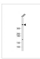
Anti-ATM Antibody (C12) at 1:500 dilution + Hela whole cell lysate Lysates/proteins at 20 µg per lane. Secondary Goat Anti-Rabbit IgG, (H+L), Peroxidase conjugated at 1/10000 dilution. Predicted band size : 351 kDa Blocking/Dilution buffer: 5% NFDM/TBST.
