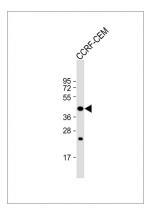
Anti-PTAR1 Antibody (Center) at 1:1000 dilution + CCRF-CEM whole cell lysate Lysates/proteins at 20 µg per lane. Secondary Goat Anti-Rabbit IgG, (H+L), Peroxidase conjugated at 1/10000 dilution. Predicted band size : 46 kDa Blocking/Dilution buffer: 5% NFDM/TBST.
