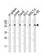
All lanes: Anti-IL2RG Antibody (N-term) at 1:2000 dilution Lane 1: human spleen lysates Lane 2: Jurkat whole cell lysates Lane 3: Daudi whole cell lysates Lane 4: KG-1 whole cell lysates Lane 5: MOLT-4 whole cell lysates Lane 6: HL-60 whole cell lysates Lysates/proteins at 20 µg per lane. Secondary Goat Anti-Rabbit IgG, (H+L), Peroxidase conjugated at 1/10000 dilution Predicted band size: 42 kDa Blocking/Dilution buffer: 5% NFDM/TBST.
