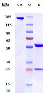
Anti-OX2R / CD200R1 Reference Antibody (Janssen patent anti-CD200R1) on SDS-PAGE under reducing (R) condition. The gel was stained with Coomassie Blue. The purity of the protein is greater than 95%
