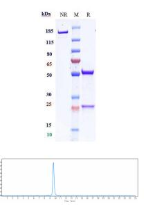
Anti-CD47 Reference Antibody (ligufalimab) on SDS-PAGE under reducing (R) condition. The gel was stained with Coomassie Blue. The purity of the protein is greater than 95%
