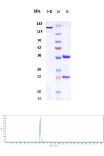
Anti-CEACAM5 / CEA / CD66e Reference Antibody (Immunomedics patent anti-CEACAM5 (Class III)) on SDS-PAGE under reducing (R) condition. The gel was stained with Coomassie Blue. The purity of the protein is greater than 90%
