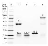
Lane 2: Reduced Rabbit IgG F(ab) Fragment (p/n 011-0105). Lane 3: Reduced Rabbit IgG F(c) Fragment (p/n 011-0103). Lane 4: Reduced Rabbit IgM Whole Molecule (p/n 011-0107). Load: 1 µg for F(ab) and F(c); 1.2 µg for IgG and IgM. Predicted/Observed size: IgG at 50 and 25 kDa; F(c) at 25 kDa; F(ab) at 25 kDa; IgM at 70 and 23 kDa. Observed F(c) Fragment migrates slightly higher.
