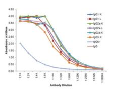
Indirect ELISA of Rabbit Anti-Mouse IgG (gamma 1, 2a, 2b, and 3) antibody. Antigen: purified mouse IgG heavy and light chains. Coating amount: 0.1 µg per well. Primary antibody: Rabbit Anti-Mouse IgG (Gamma 1, 2a, 2b, and 3) HRP conjugated Antibody. Dilution series: 2-fold. Substrate: TMB (p/n TMBE-0100).
