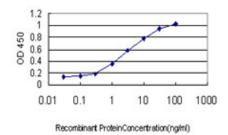
Detection limit for recombinant GST tagged IRF2 is approximately 0.1ng/ml as a capture antibody.
